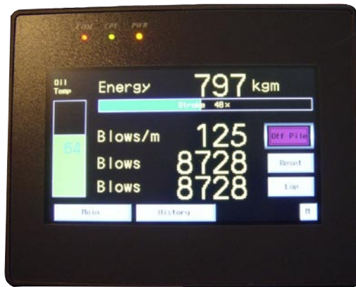
INTERFACE SCREEN MOUNTED ON POWER PACK
